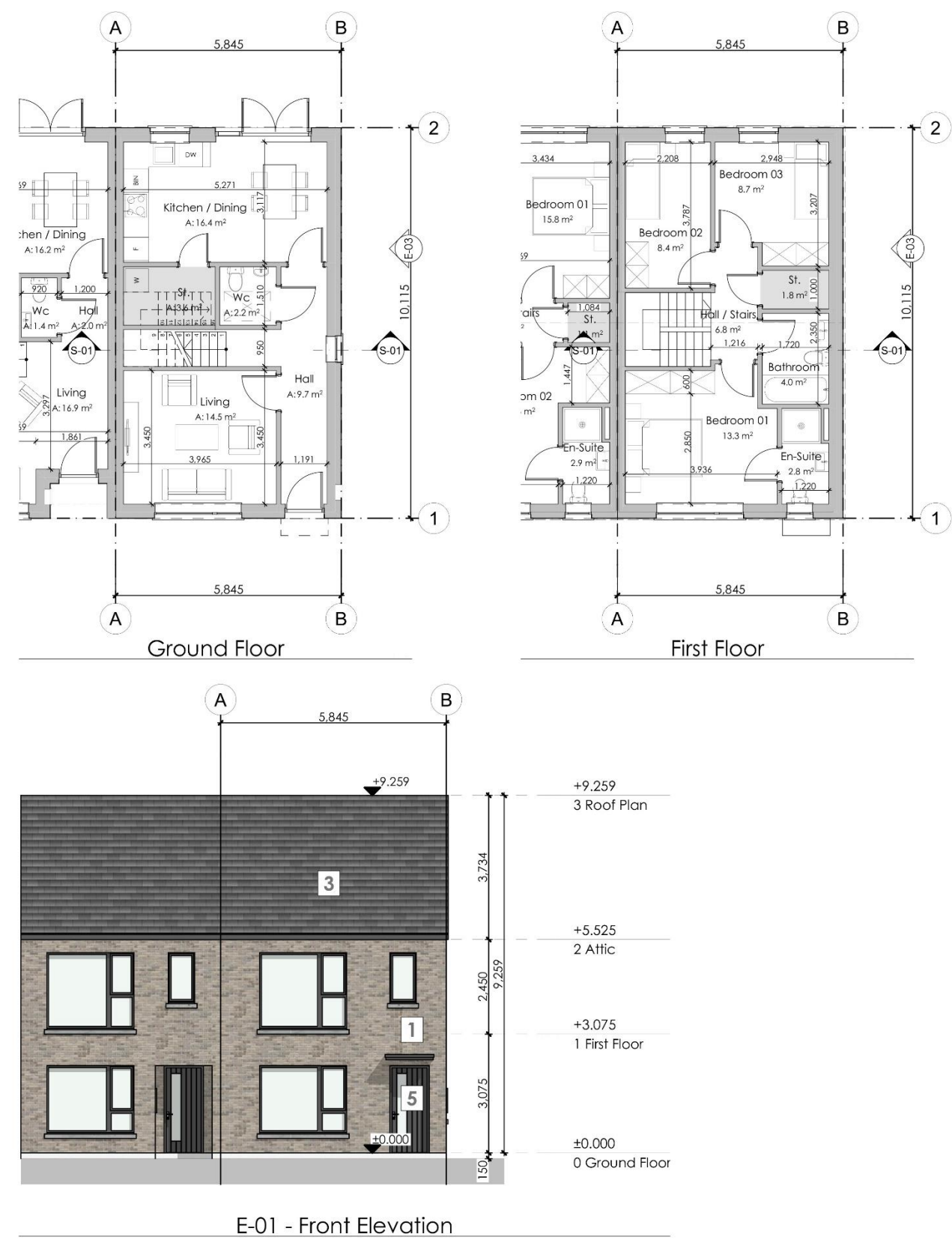
Fig 4.2 Typical house design: Plans and elevations of House Type 3.6
