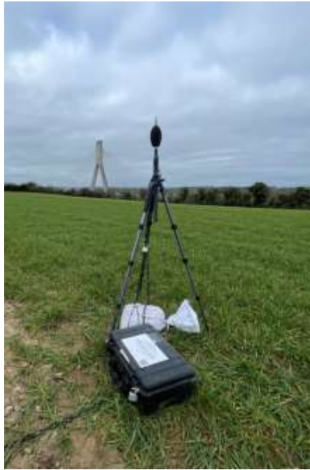
Figure 10-3: Unattended measurement setup.
