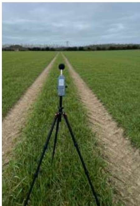
Figure 10-4: Attended Measurement Set Up
